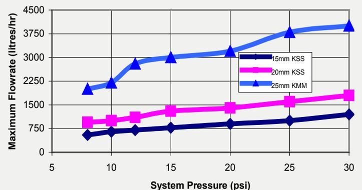
**Figure 1: maximum acceptable flow rate through KSS/KMM water meters (5 per cent pressure loss)**
