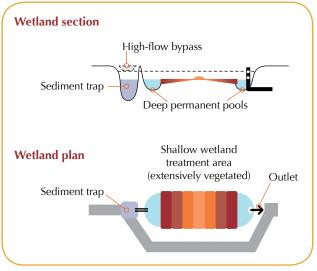
Conceptual layout of a treatment wetland showing sediment trap, high-flow bypass and deeper pools in the main wetland treatment area (Figure based on Healthy Waterways, 2006).
