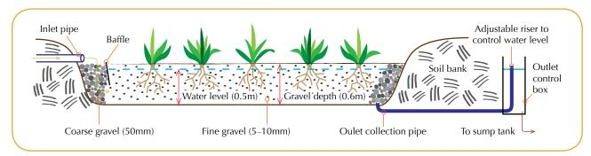
Schematic of a subsurface-flow wetland. (Original diagram courtesy of Dirou et. al, 2003).
