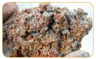
Soil mottling, above, is usually an indicator of poor drainage or water fluctuation throughout a soil profile. The dominant soil colour for this particular soil is grey. (Photo by DERM, 2007).
