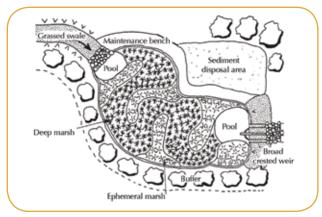
Schematic layout of a surface-flow wetland
