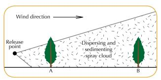
Effect of buffer distance on the point of release of the chemical
