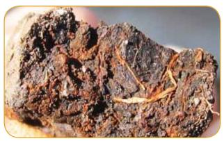
Oxidised rhizospheres (root channels), above, are thin iron deposits present in an otherwise grey matrix along small roots. (Photo by DERM, 2007).
