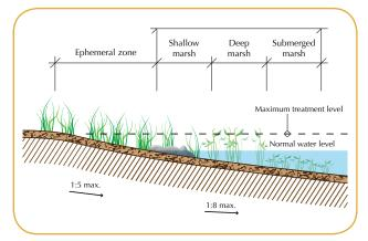
Example of bank slope and vegetation zones. (Original figure courtesy Melbourne Water).
