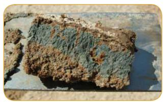
Above is a a gleyed matrix (bluish-grey or grey colour below the surface) that occupies 60 percent or more of a layer starting within 30 cm of the soil surface. (Photo by DERM, 2007).
