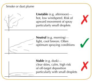
A guide to the behaviour of smoke or dust under various atmospheric conditions
