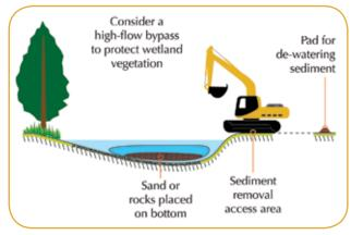
Conceptual layout of a sediment trap. (Original model courtesy Melbourne Water).
