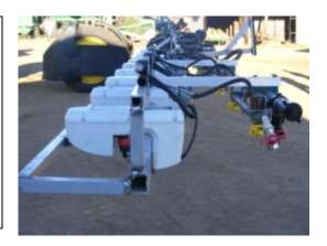
The Weed Seeker® has the ability to greatly reduce the amount of chemical applied to a paddock by detecting weeds and only spraying those areas where they are detected, hence they are operating as a spot sprayer.
