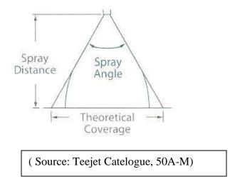
Increasing operating height will increase the sprayed width.
