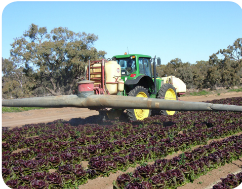
Air assisted boom in lettuce crop
