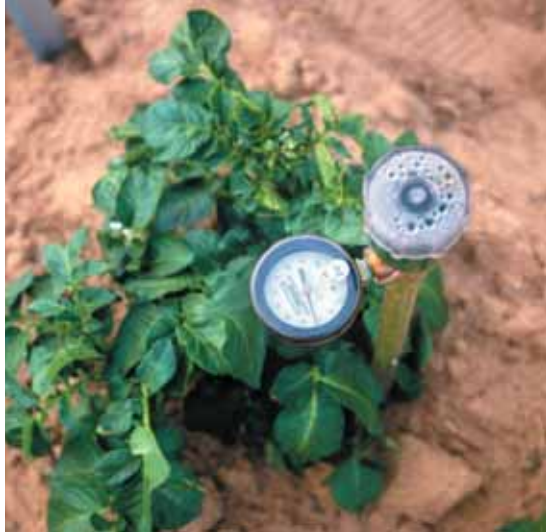
A tensiometer measures soil moisture for precise irrigation management.
