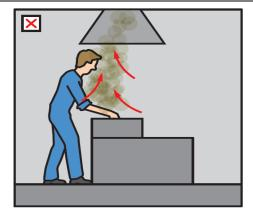
**Diagram 5:** Poor design carries contaminants through the breathing zone
