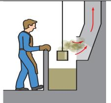
**Diagram 2:** Side hood ventilation for an open surface tank
