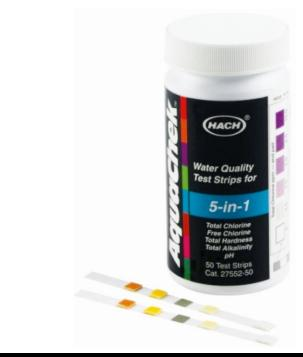
Water quality test strips can be used to assess pH and water hardness in the field. Source : Hach.com
