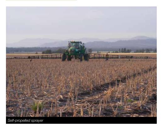
As part of the planning process, ensure that the sprayer is ready to go as soon as it is needed. This means that the sprayer and the mixing equipment are clean and decontaminated, the correct nozzles are available and calibrated, and the machine is functioning correctly.
