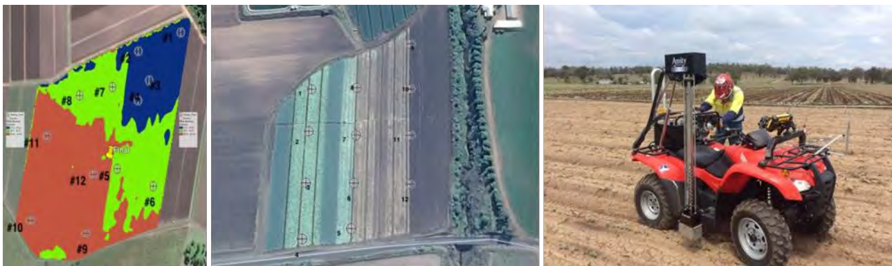
Figure 6: Soil sampling points based on EM survey perceived soil zones (left); grid-based soil sampling plan for pH (centre) and a rapid pH soil sampler mounted on a quad-bike to perform large scale pH mapping (right).
