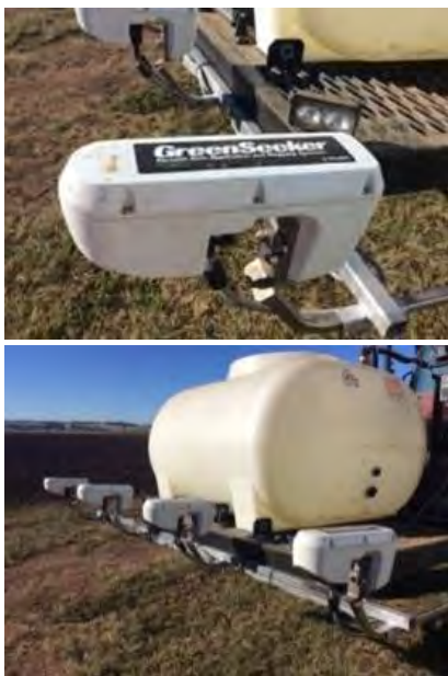
Figure 3 Greenseeker™ sensor and a 4-sensor system mounted on the front of a tractor.
