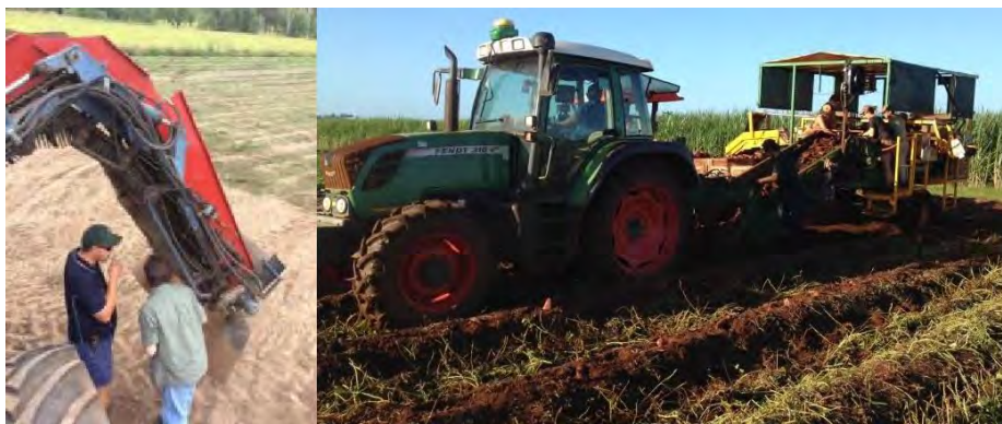
Figure 8: Kalfresh carrot harvester operator and Bernd Kleinlagel inspecting the carrot harvester's loading arm to begin installation of the load-cell based yield monitor (left) and sweetpotato harvester installed with a Greentronics yield monitor and load cells (right).
