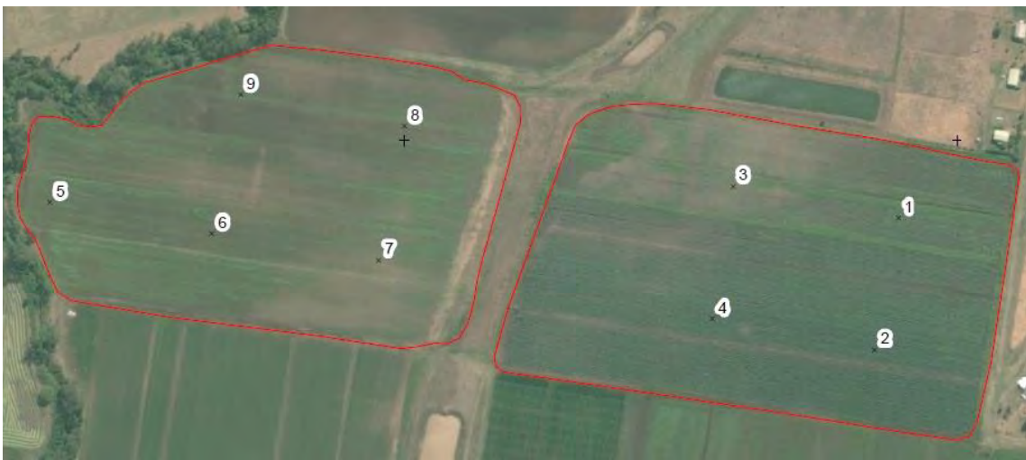
Figure 61: Grid sampling points to ground-truth EM mapping results.
