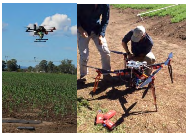
Figure 4 UAV 6 rotor craft (left), and UAV 4 rotor craft utilised to capture NDVI data through the project (right).
