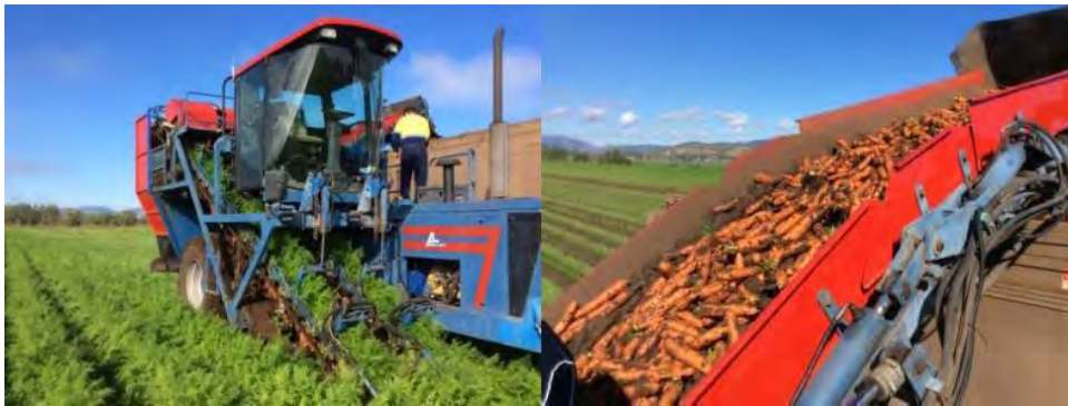
Figure 17: The mud and dirt component recorded by yield monitors of mechanically harvested carrots can be significant, up to 50% in wet conditions.
