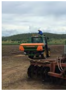
Figure 46: VRT ready granular fertiliser spreader used to deliver a VRA prescription map to Field 7.
