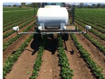
Figure 55: Tractor mounted Greenseeker crop sensors undertaking sensing (NDVI) in green beans
