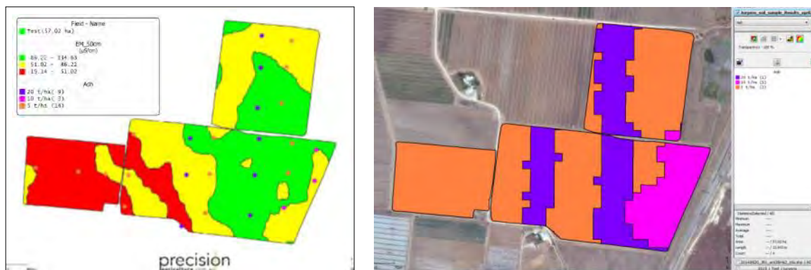
Figure 21 Compost (referred to as ash) rates based on soil test data was poorly correlated to EM perceived zones but both layers assisted agronomists and GIS specialists to meet the tomato crop’s nutrition needs recommended by agronomists (left) and final compost VRT prescription application based on soil properties and EMI mapping (right).
