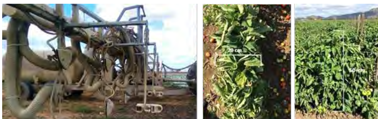
Figure 13: A six-sensor Greenseeker™ array installed at an altered angle to view the side of trellised tomatoes, left
