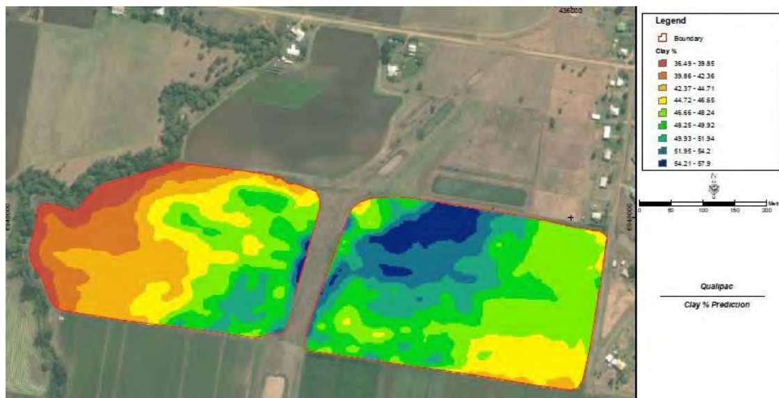
Figure 62: Clay percentage as indicated by soil texture analysis results undertaken as part of ground-truthing the EM mapping.
