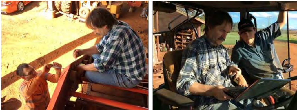
Figure 7: Producer co-operator Phil Cuda and ATV's Bernd Kleinlagel installing the load cell component of a yield monitor on a Grimme potato harvester's at Atherton (left) and ATV's Bernd Kleinlagel showing potato producer Justin Poggioli how to tare the yield monitor and interpret data from the cab-mounted control box (right) .
