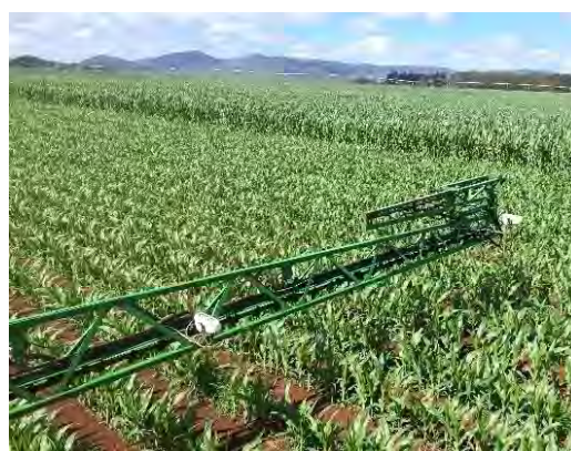
Figure 40: Greenseeker™ sensors mounted to spray boom
