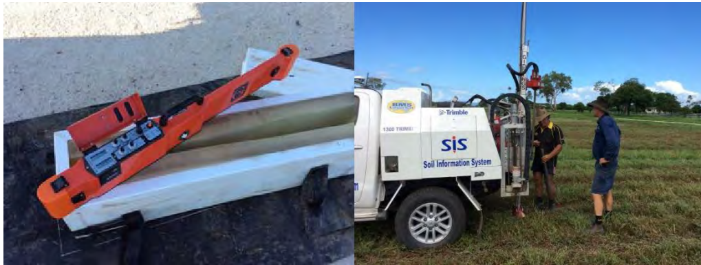
Figure 5: EM38 for rapid EMI soil surveying towed in a case by a quad-bike to survey crop-land (left) and Trimble SiS DualEM sensing and soil sampling rig.
