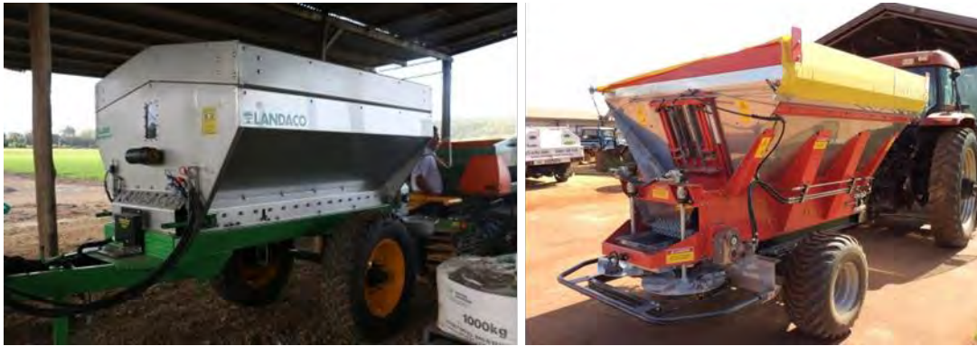
Figure 9: VR ready bulk spreader assets purchased for soil amendments in crops including sweet corn, green beans, carrots and onions, and potato production.
