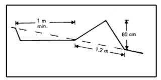
Figure 2: Cross-section of flat-channelled bank
