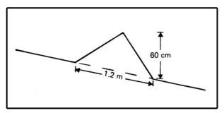
Figure 1: Cross-section of a contour bank
