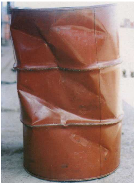
Deep dents. NOT ACCEPTABLE
