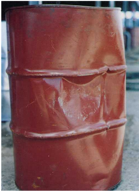
A large dent. NOT ACCEPTABLE
