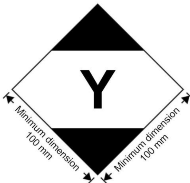
Figure 3.4.2: Mark for packages containing limited quantities conforming to Part 3, Chapter 4 of the ICAO Technical Instructions for the Safe Transport of Dangerous Goods by Air
