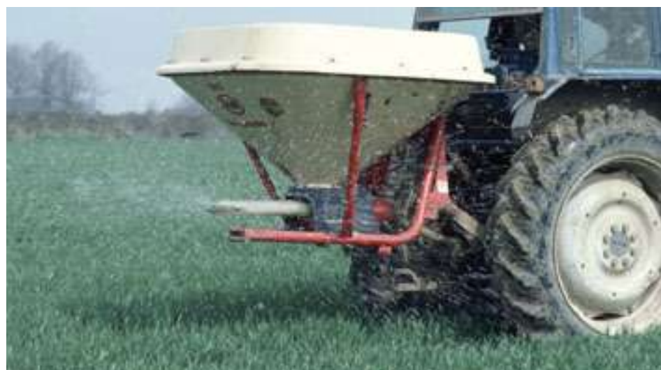
Oscillating spout spreader
