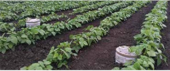
*Figure 2. Gas sampling chambers in the field on a commercial farm in the Lockyer Valley.*
