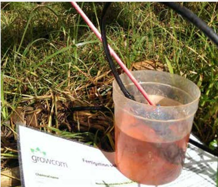
**Above: Growcom uses red food dye as a marker when conducting fertigation assessments.**
