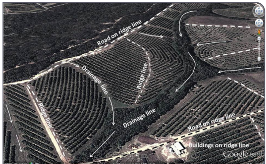
Figure 12.1: Google Earth image showing a tree mound layout on the Sunshine Coast based on subcatchments
