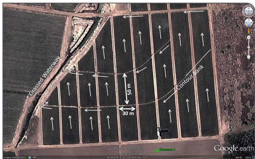
Figure 12.24: Plan view of pineapple plantation with up-and-down slope rows draining into contour banks
