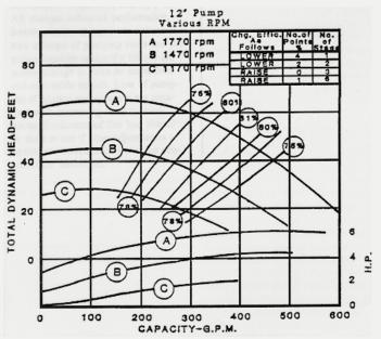
Figure 2: Example performance curve for a pump with various speeds
