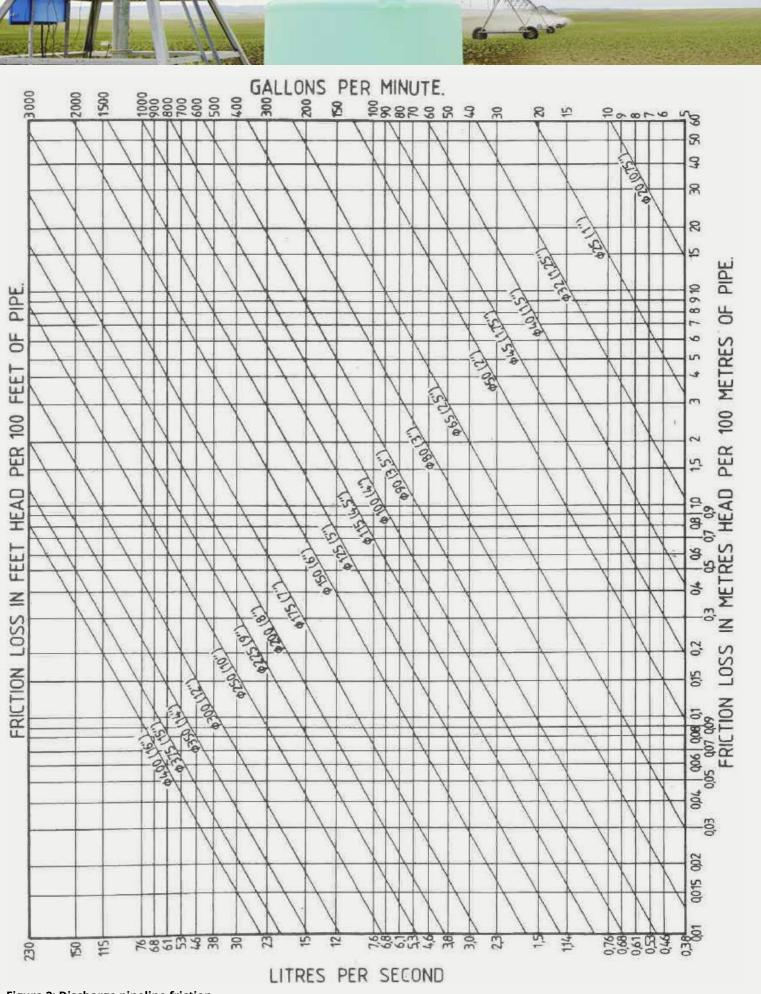
Figure 2: Discharge pipeline friction
