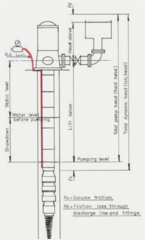
Figure 1: Total Dynamic Head Diagram
