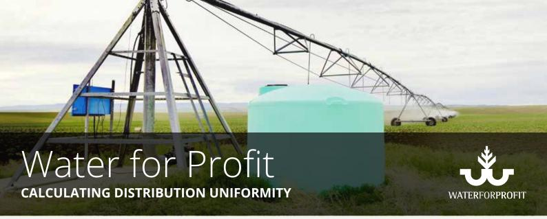
Distribution Uniformity (DU) is a key indicator of the performance of your irrigation system. DU tests should be done to ensure that your system is applying irrigation water evenly to your crop.
