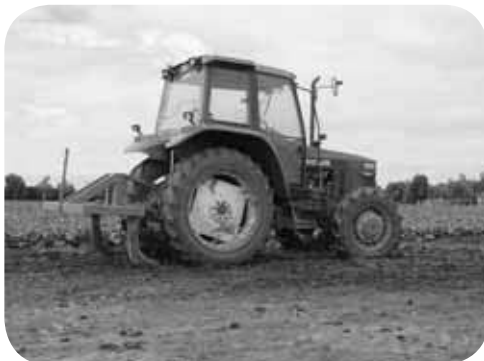
Figure 6.3 Deep rippers used to break hardpans, improving soil structure and deep drainage
