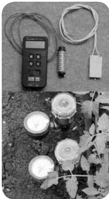
Figure 7.2 Soil moisture sensing equipment: matric and gypsum blocks and tensiometers in a tomato crop
