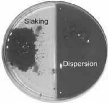
Figure 4.8 Aggregates of soil that have slaked but not dispersed (left) and slaked and dispersed (right)
