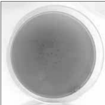
Dispersion score 4: Complete dispersion leaving only sand grains in a cloud of clay
