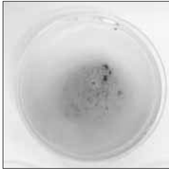
Dispersion score 3: Strong dispersion with considerable milkiness and about half of the original volume of the aggregate dispersed outwards
